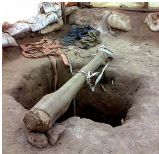
Miners use a rope attached to a beam stretched over the mouth of the pit as support to climb down into the pit or climb out. © Amnesty International and Afreewatch
